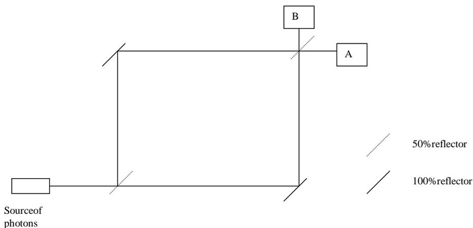
**Figure 1.** Diagram of a simple Mach-Zehnder interferometer, ignoring the thickness of the beamsplitters.
