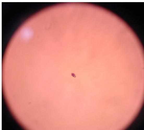
**Fig. 7.** Damage to FGB67 colored glass from exposure to  $\sim 850$  mW of unfocused 1550 nm light. Thus, the material will be feasible for future micro-object heat asymptotics research since it transmits 980 nm light and absorbs 1550 nm light.
