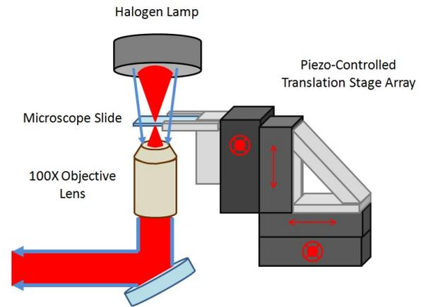
**Fig. 2.** Model of the optical tweezers system. A 100x microscope objective lens tightly focused the laser light to a very small part of a microscope slide containing a microsphere solution. The slide was mounted to a three-dimensional translation stage with a fourth piezo driven stage added for increased precision. A halogen lamp sent light back through the system to illuminate the sample on a CCD.
