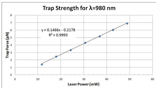
**Fig. 5.** Stoke’s drag force measurement of the trap strength for  $\lambda = 980$  nm. The trap strength increased linearly as the laser power was increased, and the trap force values were nearly identical to values measured by previous groups.
