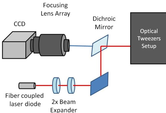
**Fig. 1.** Model of the overall optical tweezers system. A fiber coupled laser diode sent collimated laser light into a beam expander where it was directed into the optical tweezers setup by two mirrors. The optical tweezers had a halogen lamp which sent white light through the dichroic mirror where it was focused on the CCD to produce images of trapped objects.
