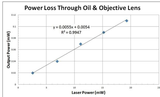
**Fig. 6.** Loss of optical power due to the objective lens for  $\lambda = 1550$  nm. The output power was reduced by two orders of magnitude. Overall, the objective lens only transmitted 0.5% of the input power.
