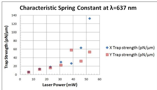
**Fig. 3.** Brownian motion measurement of the trap strength for  $\lambda = 637$  nm. The trap strength in the x and y direction is the same below 30 mW, which is an improvement to data from previous groups which showed the trap strength in the y direction as being an order of magnitude lower than in the x direction. Above 30 mW, the trap strengths vary, but this is due to the tracking software being unable to differentiate minute position changes of the microsphere at higher trap strengths.
