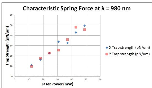
**Fig. 4.** Brownian motion measurement of the trap strength for  $\lambda = 980$  nm. Consistent with data from the Brownian motion data taken for the 637 nm trap, the trap strengths in the x and y directions were the same below 30 mW. The variance between the x and y directions above 30 mW was decreased due to refinement in batch processing.
